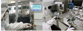
Helium leak detection
